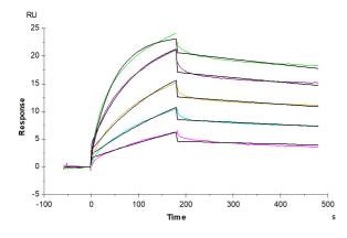
Biotinylated Human Claudin18.2 VLP captured on CM5 Chip via Streptavidin can bind Anti-Claudin18.2 Antibody with an affinity constant of 1.28 nM as determined in SPR assay (Biacore T200) (QC Test).
